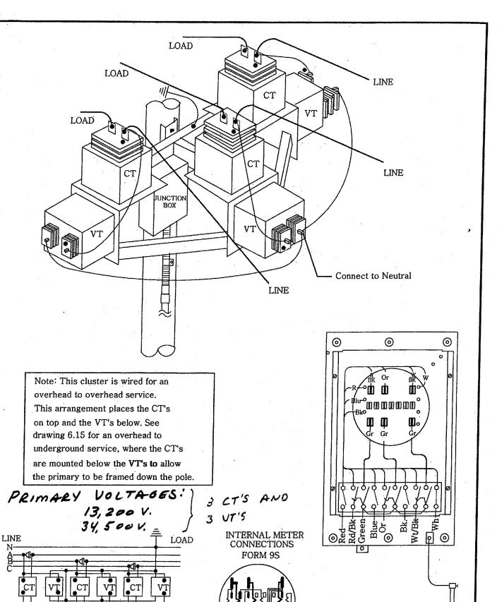
3-PHASE, 4-WIRE, PRIMARY WITH CT's & VT's FORM 9S METER, TRANSFORMER-RATED
